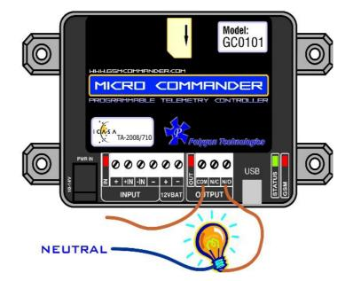
This output can be used to control devices and appliances, and is rated for 8A DC. It may be used to control most types of electrical loads, excluding AC motors above 500W.
