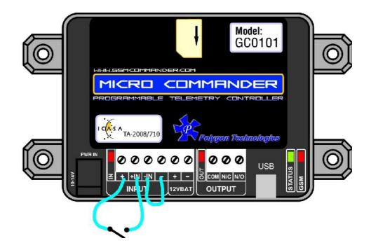
You may need an input to activate when power is supplied from some other unit. A good example will be a burglar alarm that applies power to the wires going to the siren. In such a case, it will be a simple matter of connecting the positive wire to the +IN input, and the negative wire to the -IN input.
