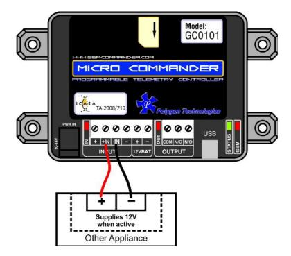
Please keep in mind that these inputs are designed for 3V to 20V operation. If you require to connect a voltage above 20V to these terminals, you should connect a resistor in series with the input, as shown below.
