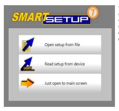
The software will show this screen when started. Here you can select whether you would prefer opening an existing setup from a file on your PC, retrieve the setup currently on the Micro Commander, just open to the main screen.
