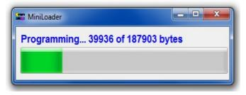
The loader utility will now show this screen, which means the firmware is being updated. The green LED, labelled "**STATUS**" on the Micro Commander, will start flashing.
