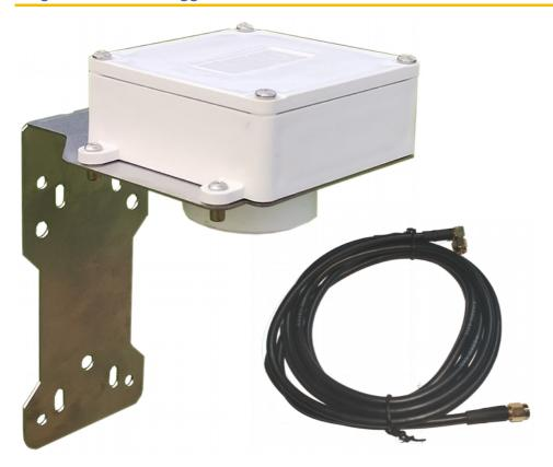
These antennas are supplied with an integral stainless steel mounting bracket and also a 2m coaxial cable to connect the SMA connector on the RemoteFloat to the SMA connector on the bottom of the antenna. For best results, the antenna should be mounted outdoors, as high as possible.
