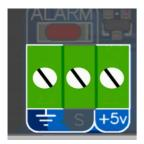
The PumpStation can be powered from a 5V DC voltage source, and shares a ground connection with the alarm output.
