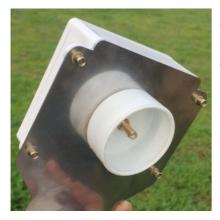
At the bottom of the antenna is a round PVC 50mm fitting, where standard 50mm PVC waste pipe can be slotted in, in order to provide protection for the coaxial cable in environments where baboons are a concern.
