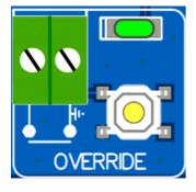
The TankStation has an override button and input. The input is activated when the two terminals are connected to each other. The button is physically wired across this input, so that pressing the button has exactly the same effect as connecting a wire across the two terminals.
