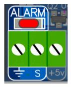
The device has an open-collector alarm output. This can be used to drive an input on a GSM Commander or provide local indication via a buzzer or LED.. When active, an
